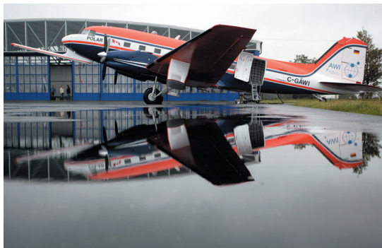
▲ 'Polar 5' with geophysical booms and antennae in front of hangar 5 at the Bremerhaven regional airport (photo: G. Schläger)
