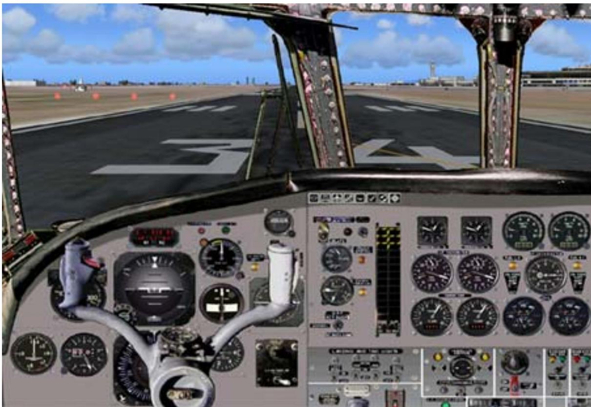
The main panel has three main parts : the pilot instruments on the left, the engine instruments on the right, and some pedestal instruments on the bottom right.
