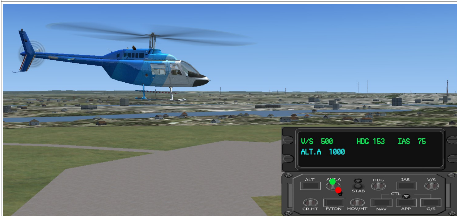
Fig. 5 – Over 40kts IAS, the HAP-gauge automatically switches to FLIGHT_MODE. - Setting VS=500 ft/min, IAS=75 kts.
