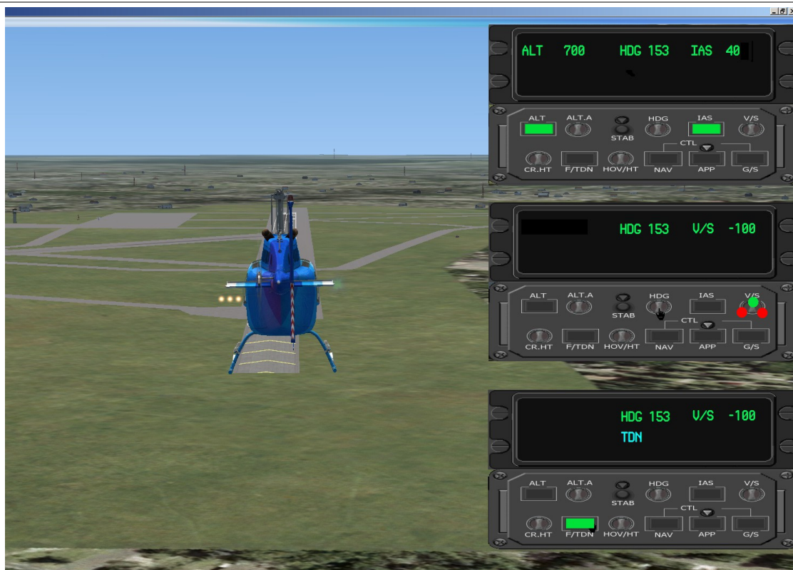
Fig. 15 – Reduce your horizontal speed to 40 kts (this is the minimum IAS in FLIGHT_MODE). Press the [CTRL][SHIFT][L] to reduce the IAS setting on the HAP-gauge.
