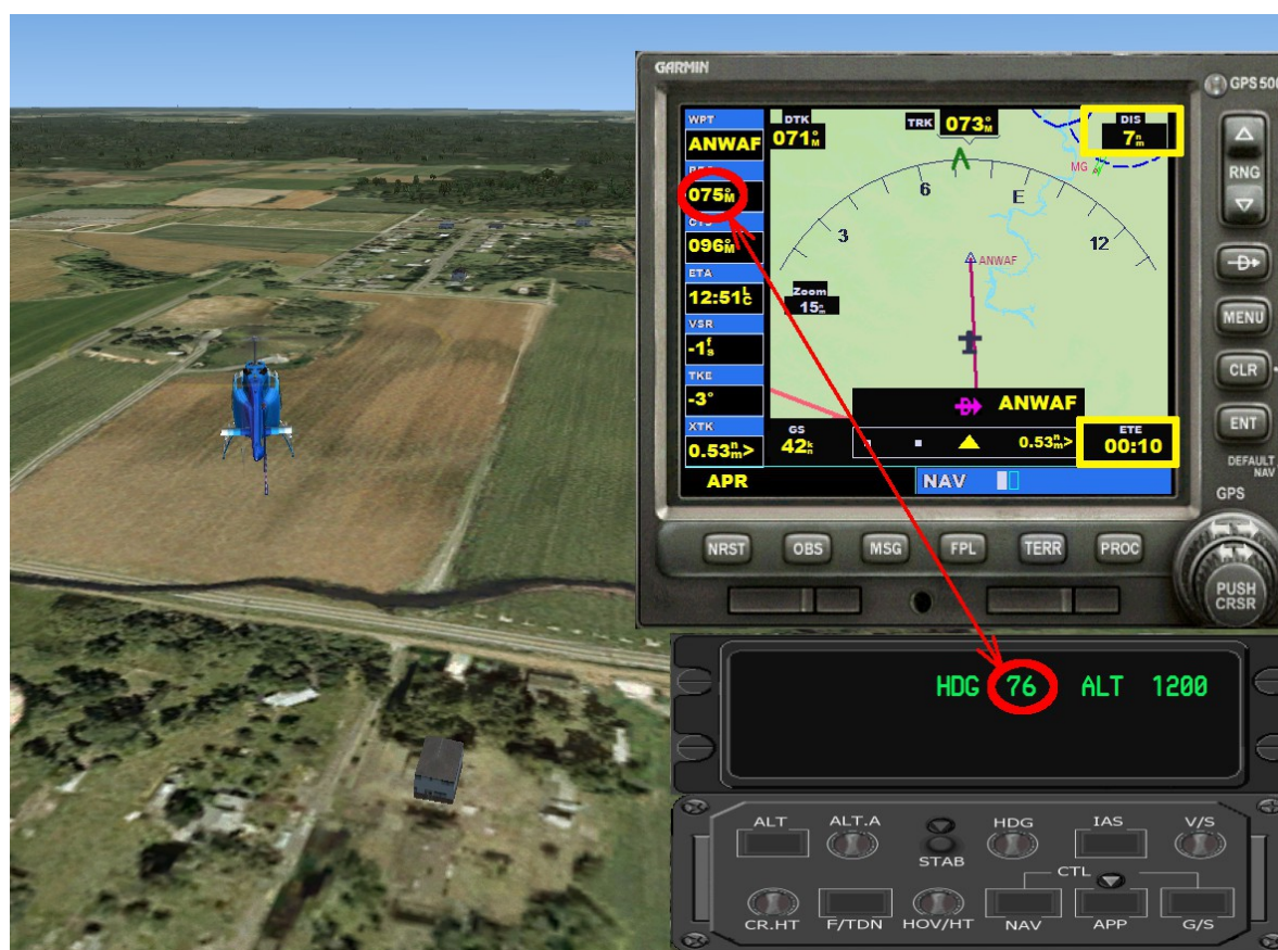
Fig. 19 - Now use the GPS function to monitor: (upper right corner, yellow square) → distance to the waypoint → 7 Miles out. (lower right corner, yellow square) → “the flight time” based on current air-speed → 10 Minutes to waypoint.
