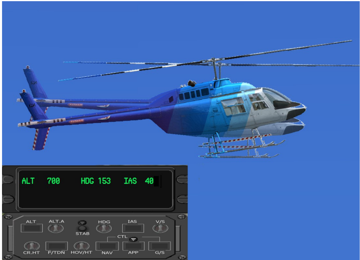
Fig. 15 – Reduce your horizontal speed to 40 kts (this is the minimum IAS in FLIGHT_MODE). Press the [CTRL][SHIFT][L] to reduce the IAS setting on the HAP-gauge.
