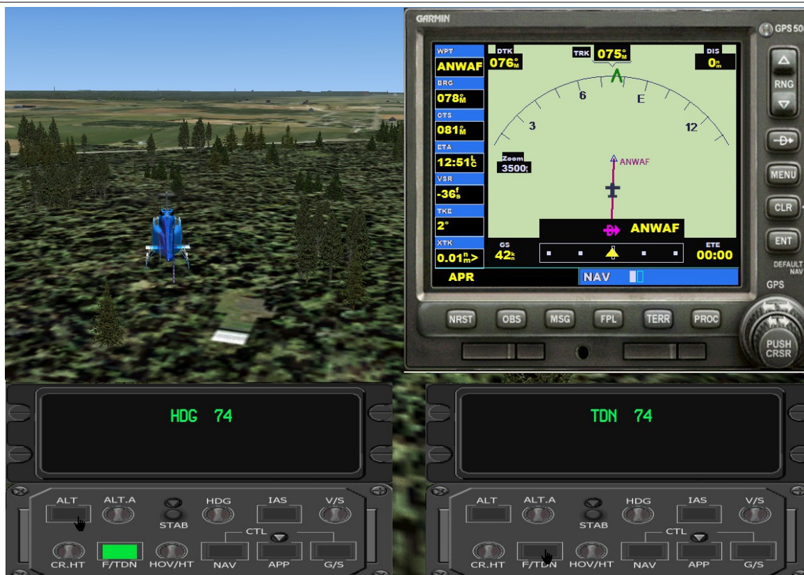
Fig. 20B – Reduce [IAS] to down to 40 kts, to make the switch to HOVER_MODE smoothly.
