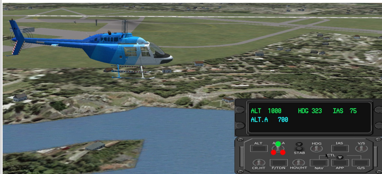
Fig. 10 - Descending to 700ft on “the downwind leg”. Turn on [ALT.A] (green spot) and set the new altitude (red spots) to 700ft.
