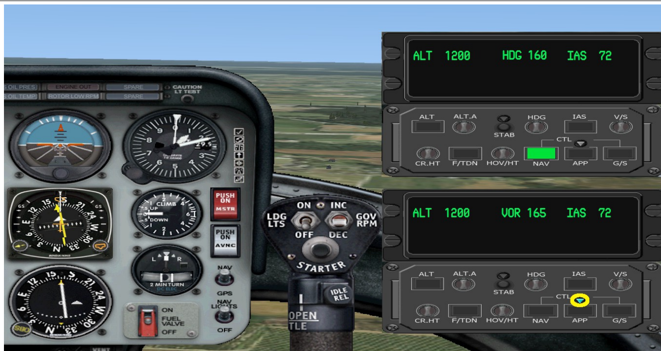
Fig. 10 – Press [NAV] to tell the HAP-gauge to fly directly to MGM-Vor.
