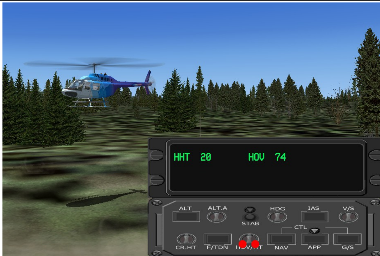
Fig. 22 – HOVER_MODE Engaged - SET [HHT] = 0 to land the helicopter on the ground.
