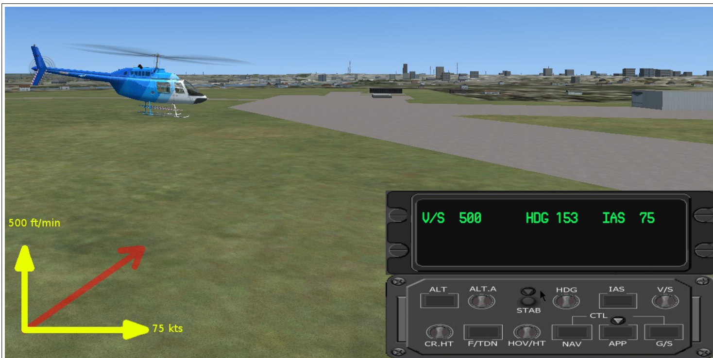
Fig. 5 – Over 40kts IAS, the HAP-gauge automatically switches to FLIGHT_MODE. - Setting VS=500 ft/min, IAS=75 kts.
