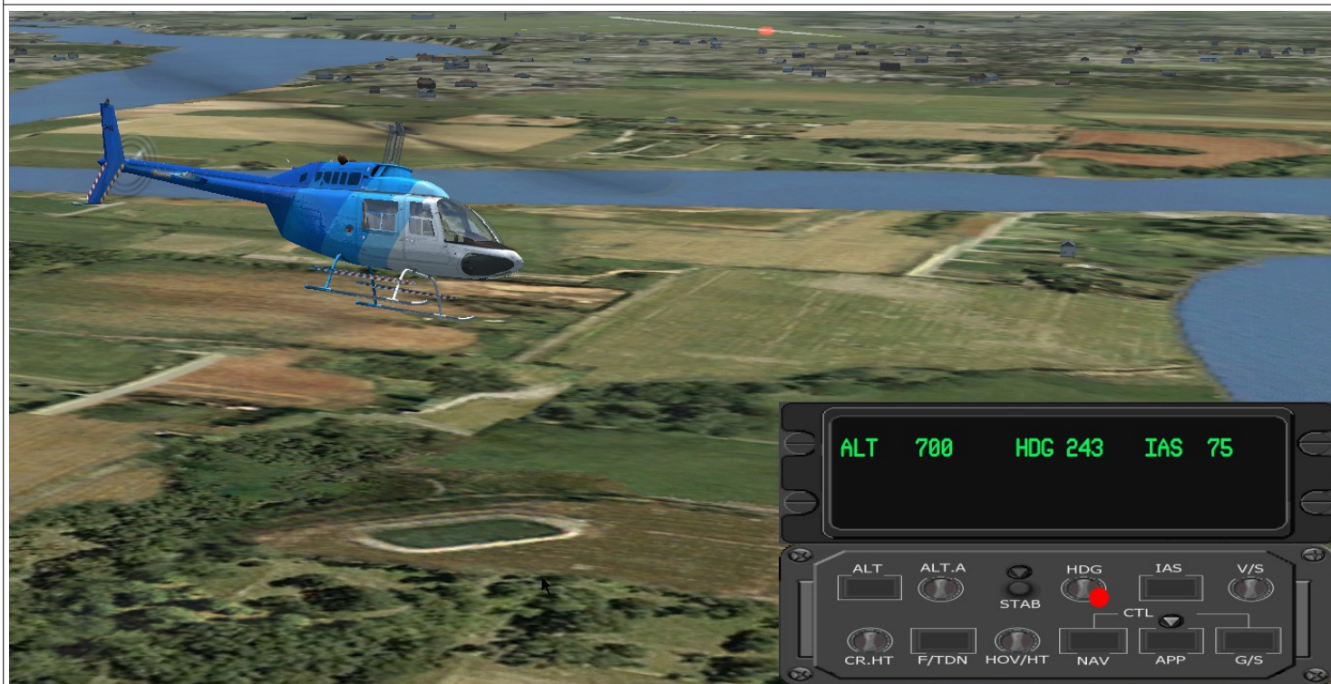
Fig. 11c - Turn ON [V/S] (green spot) and adjust V/S to -100 ft/min (red spot).
