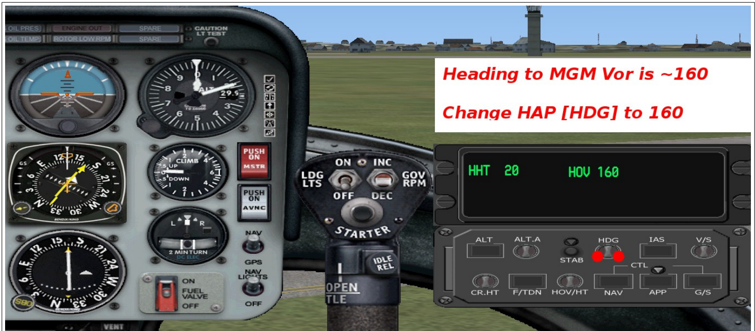
Fig.6 - Set [HDG] to 160 before take off.
