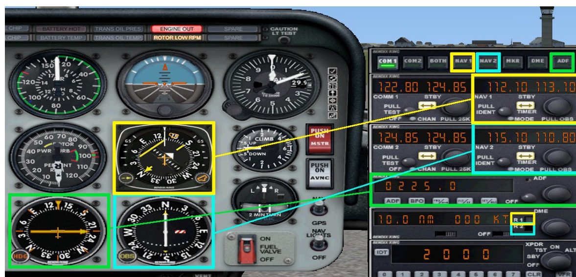
Fig 4. Which radio is connected to which instrument overview
