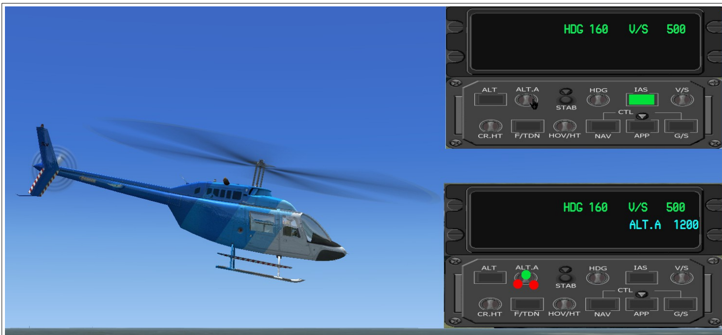
Fig.8 – When the forward speed > 40 Kts, HAP sets V/S= +500 and IAS = 75 kts automatically!
