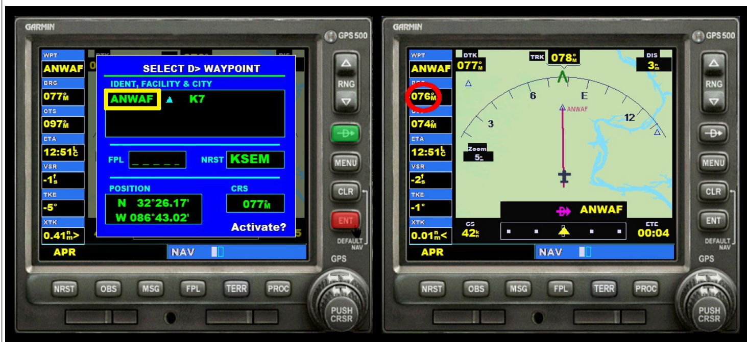
Fig. 18a – (mid) Press [DCT] (green square) on the GPS.
