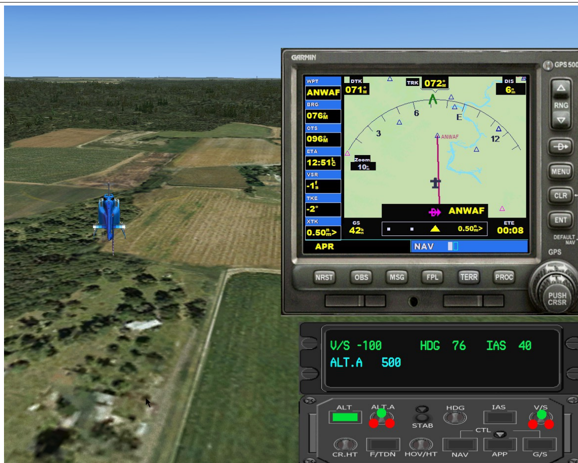
Fig. 20a – Set [ALT.A] to 500 ft and V/S to -100 to slowly descent before hovering.
