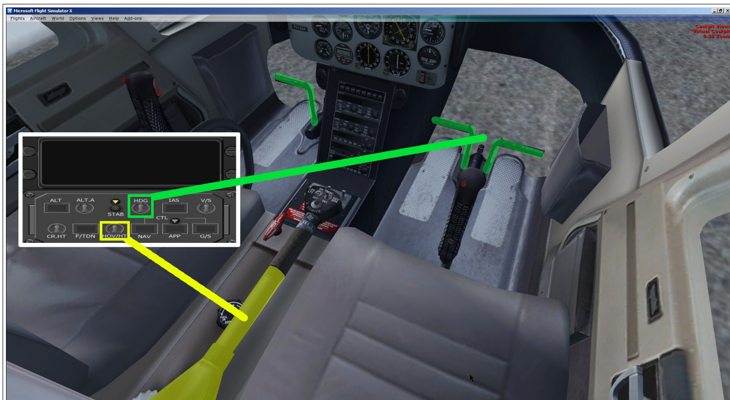
Fig. 11 - Relation between the HAP-gauge and BELL206B flight controls (Yoke, Collective Liver)
