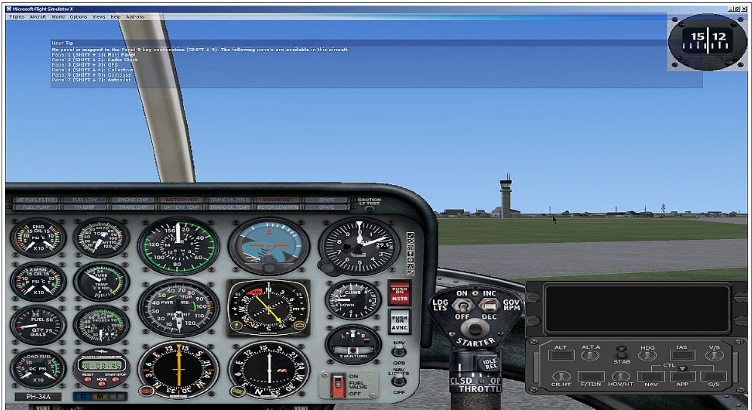
Fig. 4 – 2D panel with Collective liver, Throttle, Compass and HAP gauge
