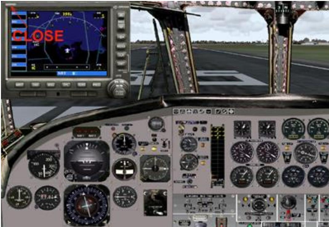
You can close the GPS panel by clicking on its SimIcon, or on the top left corner of the GPS, on the GARMIN name.
