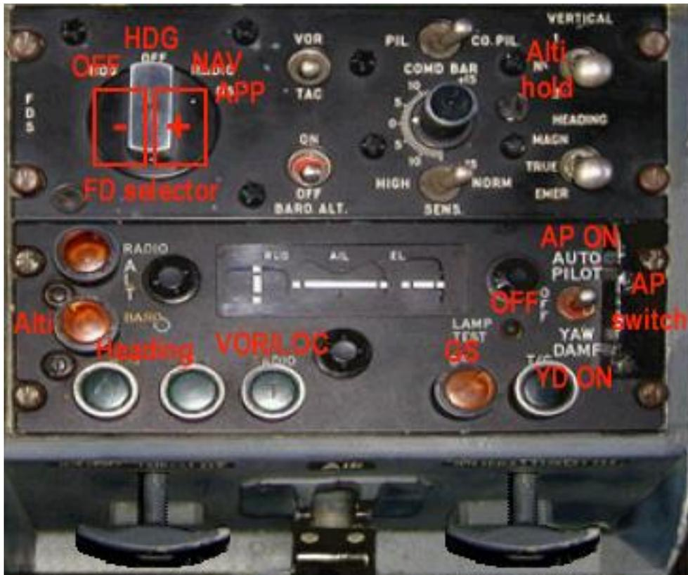
The Flight Director selector is also the FD switch ; Click on the right side of the selector button to turn it right, on the left side to turn it left. From left to right, the functions are marked as follows :
