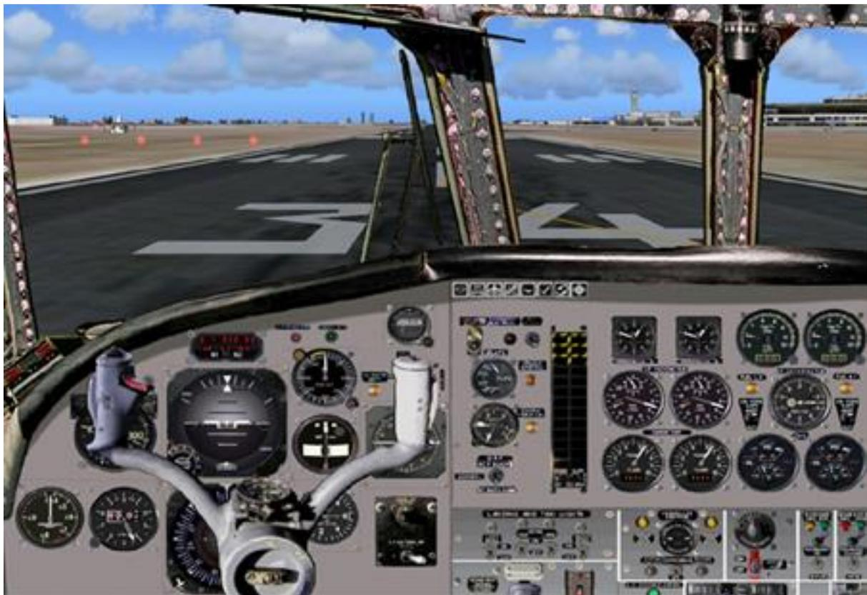
The main panel has three main parts : the pilot instruments on the left, the engine instruments on the right, and some pedestal instruments on the bottom right.
