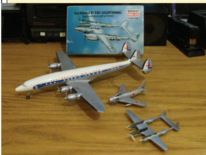
Photo 4 The Connie’s vertical stabilizers are scaled up from those of the P-38.
