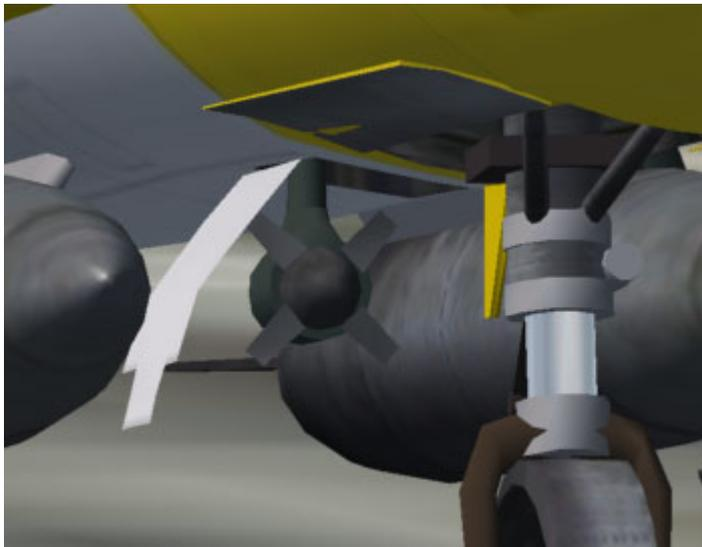
The Emergency Power Unit (EPU) consists of a small ram-air turbine connected to an alternator and a hydraulic pump. The EPU will deploy automatically if/when hydraulic pressure drops. It is retracted as soon as the engine starts.
