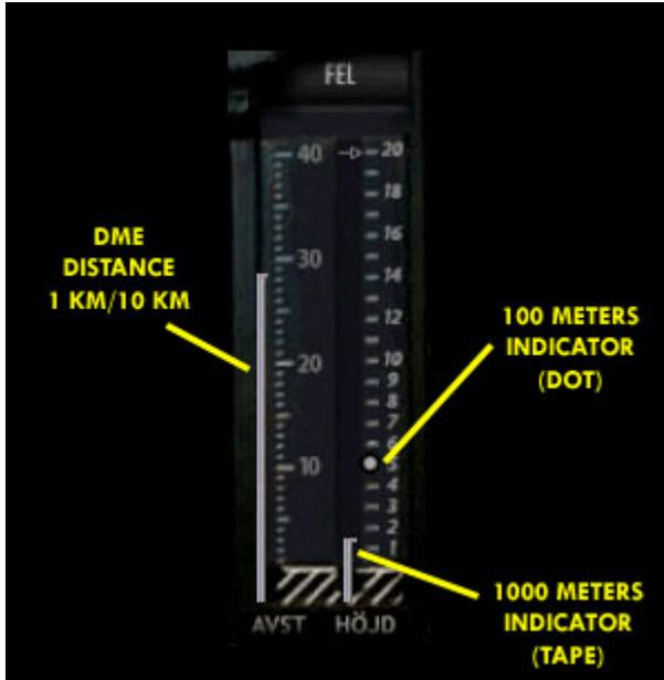
The left scale shows DME distance in ranges 0–40 km or 0–400 km, depending on the setting of the FD Mode Selector on the [PN59 Panel](#). The tooltip also shows the distance in nautical miles.
