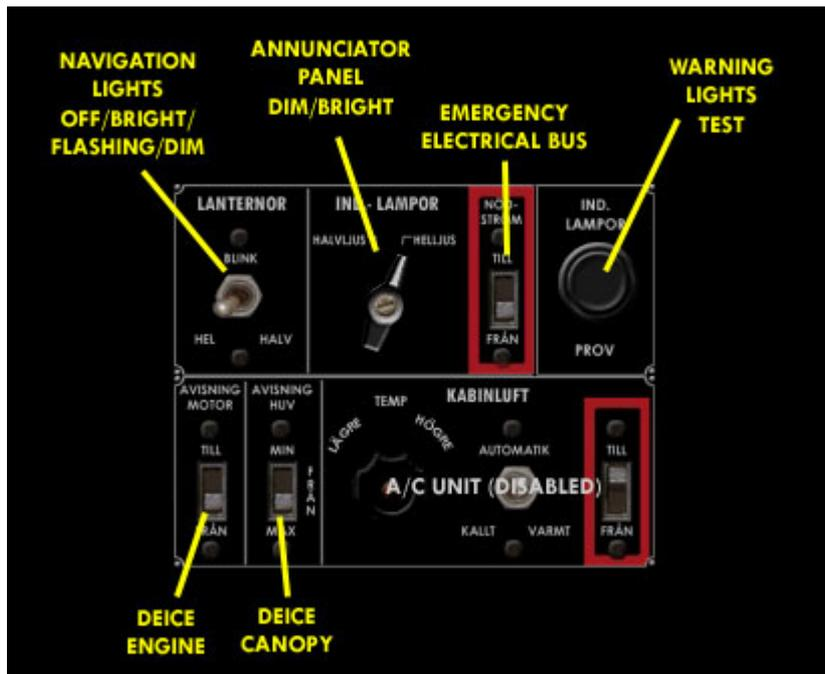
The Navigation Lights are operated by a four-way switch. Center position is OFF, HEL means bright, HALV means dimmed, BLINK means flashing.
