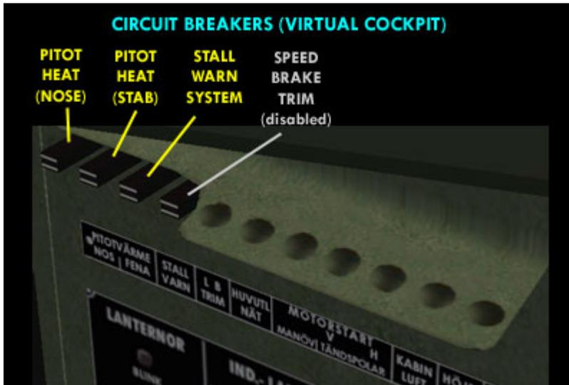
The circuit breaker panel is only visible in Virtual Cockpit view. The first four circuit breakers are used as switches for pitot heating, and for the stall warning and speed brake trim systems. All circuit breakers should be ON in flight.
