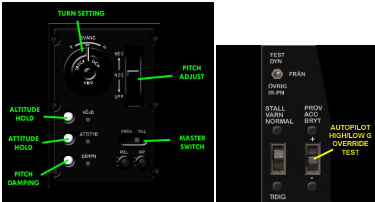
The autopilot in J 35J is **quite** different from the standard FS9 autopilot. To begin with, the master switch is sealed in the ON position, and should only be switched off in an emergency. You fly manually in the default mode DÄMPN, and the other two modes (HÖJD, ATT) use custom functions for altitude and attitude hold.
