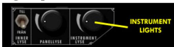
Instrument, panel and interior lights are controlled with two rheostats and a toggle switch in the left part of the cockpit. In this panel version, only the Instrument Lights control is functional, and it only has two positions: On/Off.
