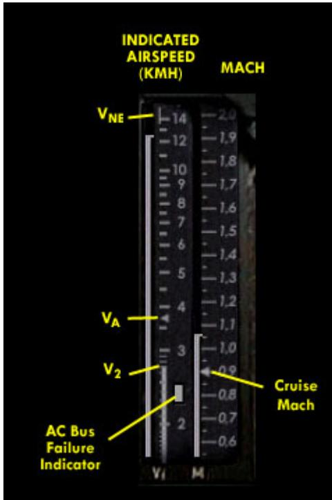
The left tape shows indicated airspeed in kilometers/hour. The right tape shows Mach number. As with most other instruments, the tooltip shows the reading in both metric and US units.
