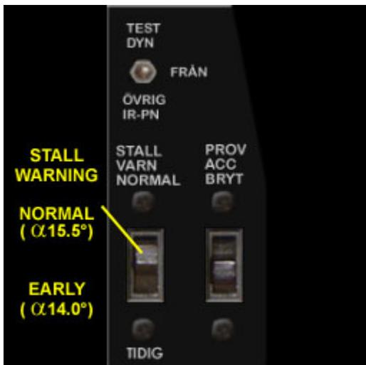
The Stall Warning System has two modes: Normal and Early (TIDIG). In Normal mode, the stall warning alarm will start rattling at 15.5 degrees alpha (angle of attack). In Early mode, at 14 degrees.
