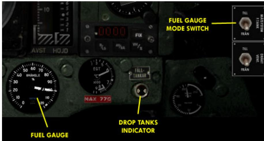
The J 35J has two main sets of tanks, forward and rear, holding 1430 litres each. Four external (drop) tanks with 525 litres each can be added, two under the fuselage and one on each outer wing pylon, giving a maximum of 4960 litres. The default configuration in this model is one pair of drop tanks.
