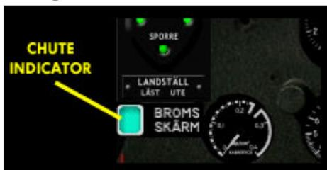
The Drag Chute Indicator has three positions:
