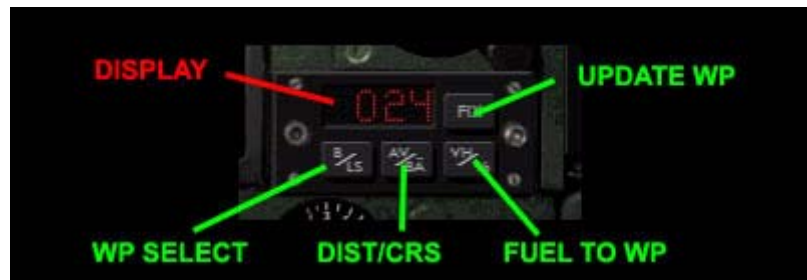
Fig. 15 FLI 35 Indicator Unit
