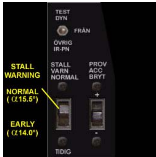
Fig. 36 Stall Warning System
