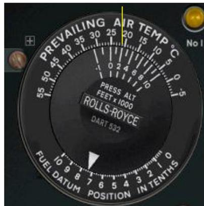
In this example the airfield pressure altitude is 2000ft. The ambient temperature is 21°C. The computer shows the correct trim setting is 74%.
