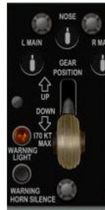
The Undercarriage Selector is to the right of the engine instruments and a standard six lamp position indicator is fitted beneath.
