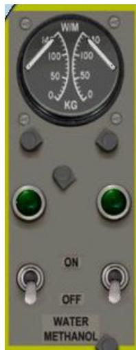
The pumps are controlled by two switches on the starboard overhead panel. The green warning lamps indicate sufficient system pressure. A W/M contents gauge is positioned above the lights, clicking on its face while the aircraft is on the ground will replenish the tanks. Each tank has a maximum capacity of 140 kg.
