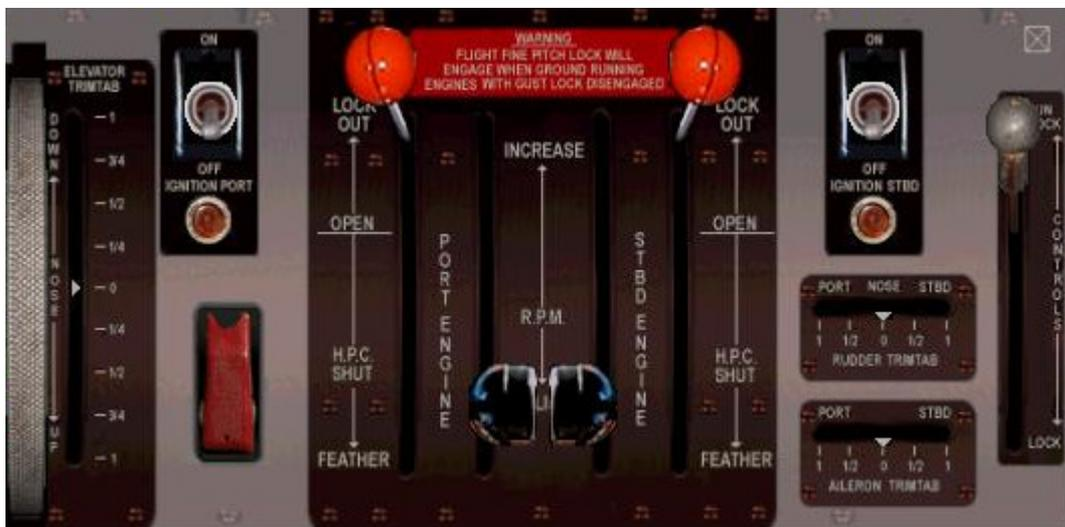
Outboard of the throttle levers are two high pressure (HP) fuel cock levers, each having **four**/three positions. The functions of each position from fully forward (default) to fully rearward are: **(Red text not applicable to Dart 6 engines)**
