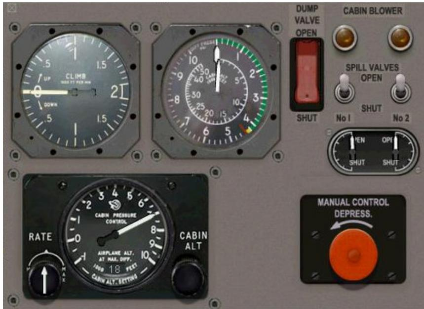
The controls for the pressurisation system are grouped on the co-pilots side panel and consist of a Dump Valve switch, two Spill Valve switches and associated position indicators, two Blower Failure red lamps, a pressure controller, and cabin height, pressure differential and rate of climb indicators. A manual depressurising valve is also provided.
