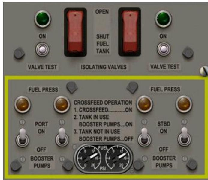
The fuel tanks can be isolated by means of two guarded switches on the starboard overhead panel which control a valve between the fuel tank and collector tank. Test Switches and associated green warning lamps allow testing of the valve circuit.
