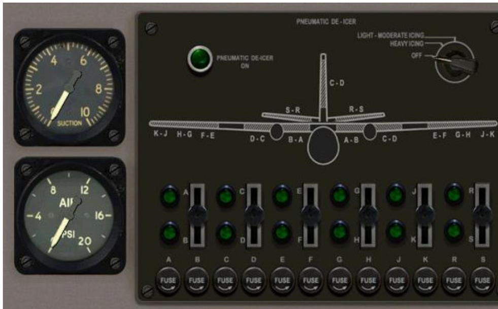
The rotary switch has three positions OFF/HEAVY ICE/LIGHT ICE. A green Pneumatic Deicer On lamp will light with the system selected on, and a set of green lamps representing the sections of the system will light cyclically as each section is inflated. Spring loaded Manual Override switches enable any section of the system to be manually operated.
