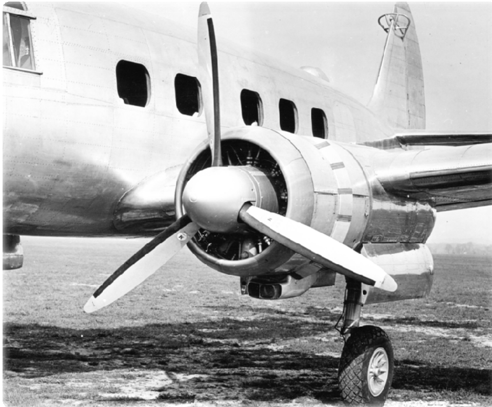
Close up shot of port side Alvis Leonides on the prototype Y-0222.
